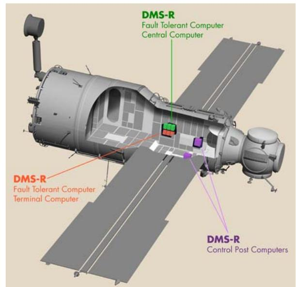
The European developed Data Management System (DMS-R) computer provides Command and Control for Zvezda and the entire Russian segment of the International Space Station. In addition it provides Guidance, Navigation, Control and mission management to the whole station. (Image: ESA/D. Ducros)
