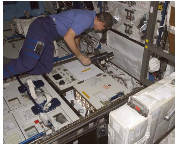
Maintenance Operations: Expedition 12 Commander Bill McArthur preparing to remove the Avionics Air Assembly from the Crew Health Care System (CHeCS) rack on 9 December 2005. (Image: NASA)
