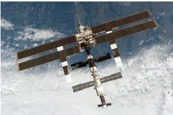
Photo of ISS taken during the STS-114 mission on 6 August 2005. Solar arrays are clear to see running in approximate left to right direction. Two sets of radiators that form part of the thermal control systems are clear to see running underneath and perpendicular to the largest set of solar arrays. (Image: NASA)
