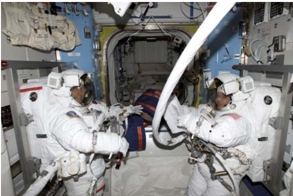
Astronauts Carl Walz (left) and Daniel Bursch, Expedition Four flight engineers, undergo a pressure check in Quest's Equipment Lock, prior to the beginning a five-hour, 47-minute EVA. (Image: NASA)
