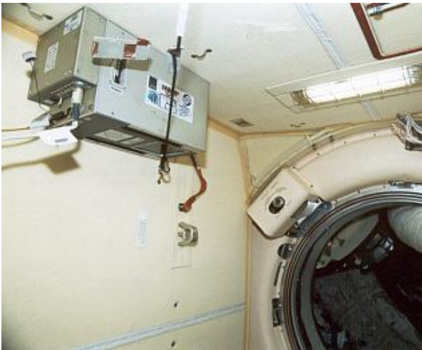
AST/Sileye-3 cosmic ray detector shown in the Pirs Module on the ISS.
