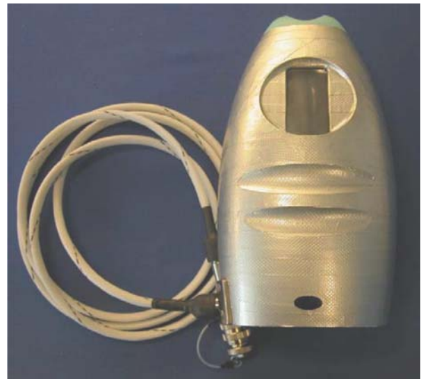
Platon Device, the Nitric Oxide detection hardware used in the NOA experiments. (Image: ESA)
