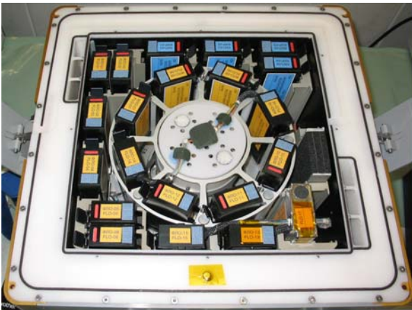
Example of Kubik incubator with centrifuge configuration loaded with experiment containers. (Image: ESA)
