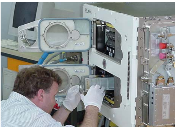
ESA astronaut Reinhold Ewald inserting an experiment container into the EMCS Engineering Model. (Image: ESA)
