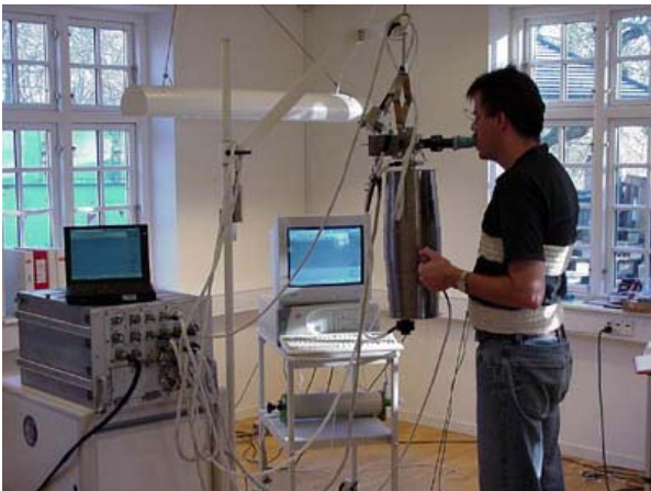
The ESA-developed PFM/PAM units for the Pulmonary Function System in operational mode
