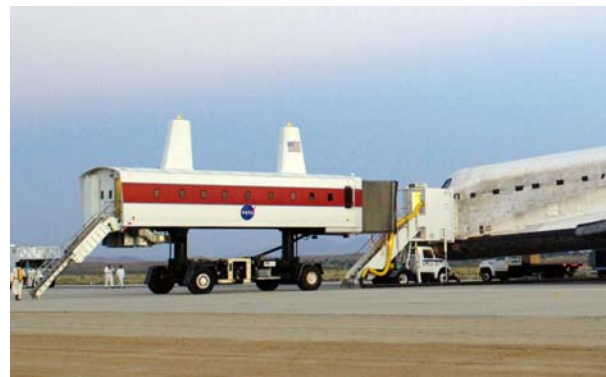
Crew Transport Vehicle pulls up to the Space Shuttle Discovery to offload the crew following landing of the STS-114 mission. 9 August, 2005. (Image: NASA)
