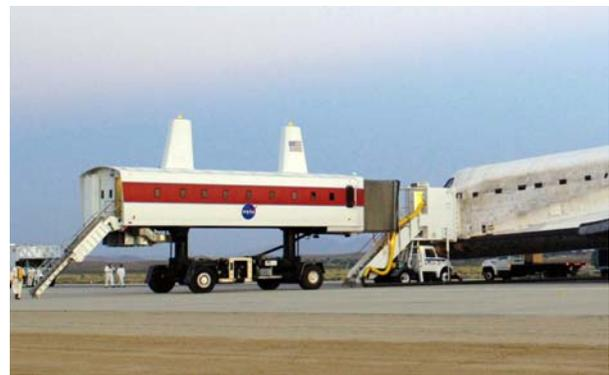
Crew Transport Vehicle pulls up to the Space Shuttle Discovery to offload the crew following landing of the STS-114 mission. 9 August, 2005. (Image: NASA)
