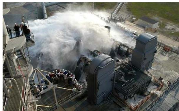
Sound Suppression System test on launch pad 39A at the Kennedy Space Center. (Image: NASA)
