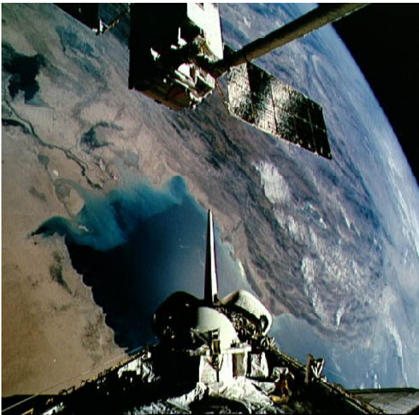
ESA's European Retrievable Carrier (EURECA) being held by the Shuttle's robotic arm prior to deployment on STS-46 Shuttle mission in 1992. (Image: NASA)
