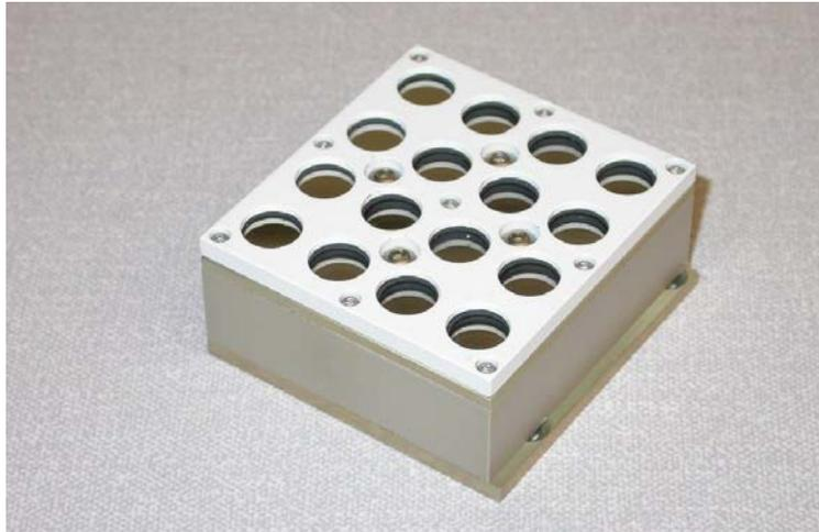
PHOTO-I experiment hardware, which will contain unicellular algae
