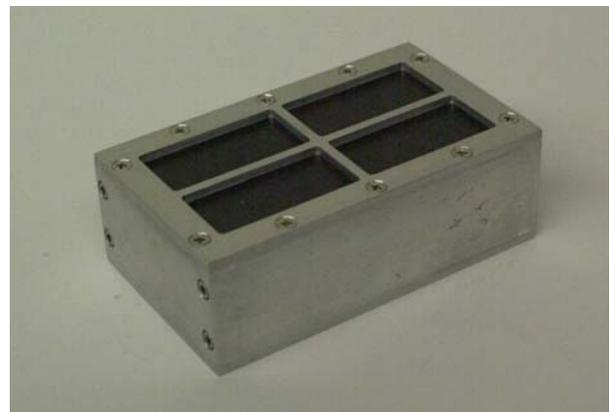
LETVAR experiment hardware, which will contain four different types of shielding material
