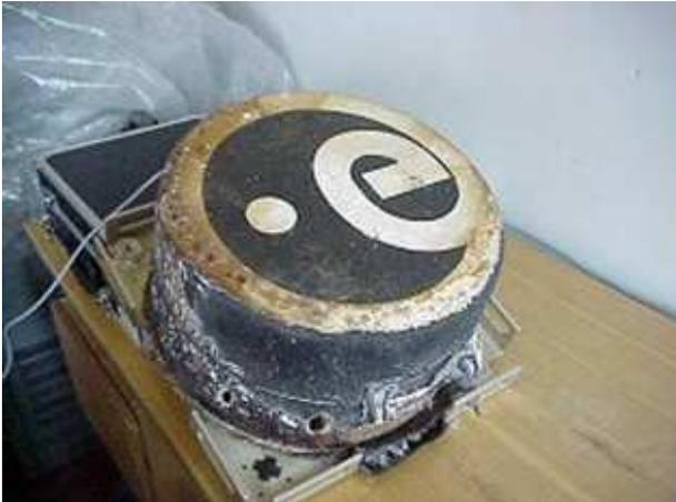
Biopan after landing with the lid closed. The facility is covered by a massive ablative skin to shield the experiments against the re-entry heat.
