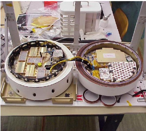
Biopan before flight at ESTEC, with the hinged lid open. Experimenter-provided packages are mounted on support plates in the bottom and the lid. (Image: ESA)
