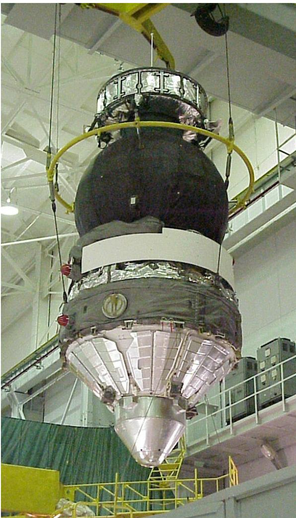
Closed Foton-M1 spacecraft during procedures to integrate it into a Soyuz launcher nose cone in 2002. (Image: ESA)
