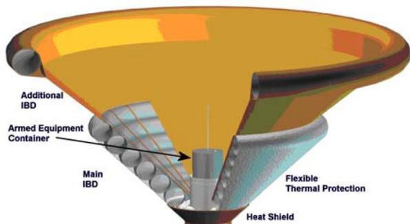
Cut out artist's impression of IRDT with flexible heat shield and inflatable extension deployed (Image: ESA)
