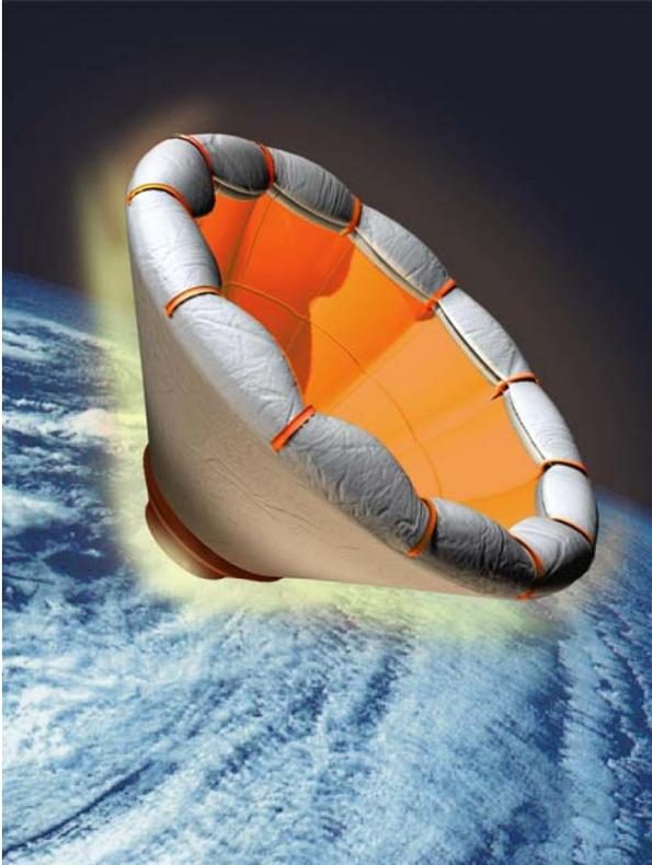
Artist's impression of IRDT entering Earth's atmosphere with flexible heat shield deployed (Image: ESA)
