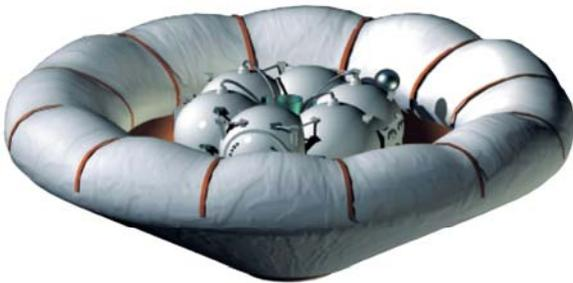
Soyuz Fregat upper stage entry configuration with IRDT flexible heatshield deployed (Image: ESA)
