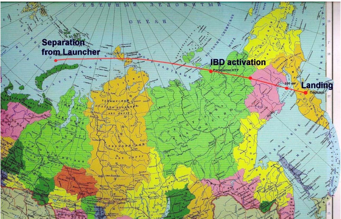
Ground track of the IRDT following separation from the launcher (Image: ESA)
