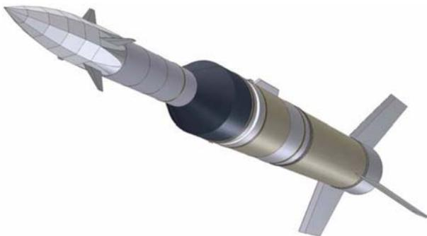
*Figure 9: Planned SHEFEX 2 re-entry vehicle using a more powerful rocket configuration consisting of the Brazilian motors S40 and S44. Credits: DLR*
