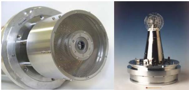
Figure 1: ECOMA Particle Detector for Meteor Grains (left) and a Combined Sensor for Neutrals and Electrons (CONE). Credits: IAP
