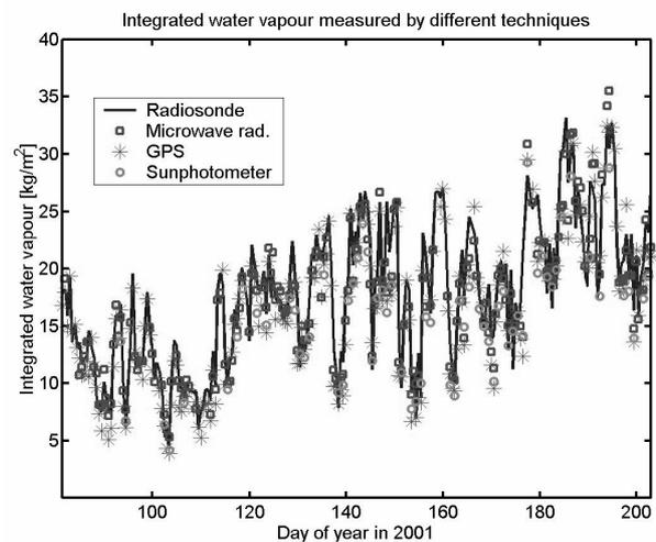
Figure 4 – Integrated water vapour (IWV) measured over a three month period at the University of Bern using the sun photometer, TROWARA microwave radiometer and Global Positioning System (GPS) receiver.
