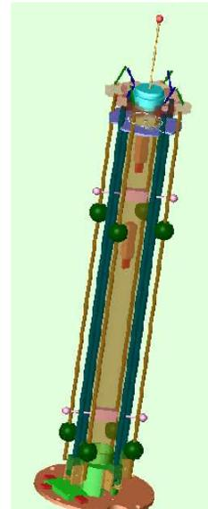
Figure 2. The payload of 21.131 consisted of a spherical (tip) and a ring (blue cylinder) Langmuir probe, an impedance probe with transmitter and receiver dipoles located just below the ring LP and near the base of the central tube, and E-field detectors (green spheres) mounted on folded booms shown here in the stowed configuration.
