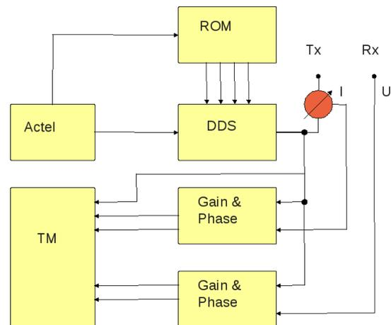
Figure 3. Schematic of Impedance probe design.
