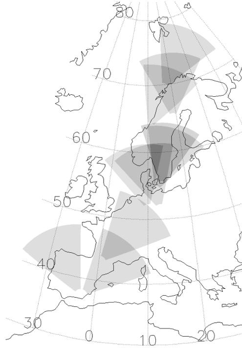
Figure 2. Overview of the IAP NLC camera network. Grey shaded areas show the field of view of each camera projected to the altitude of 83 km. The cameras can observe NLC from  $38^\circ$  N to nearly  $80^\circ$  N.
