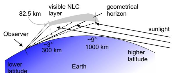
Figure 1. Noctilucent cloud observation geometry. The clouds become visible when the sun is below the horizon but still illuminating the clouds. If the upper cloud limit is observed at 12° elevation the cloud edge is located about 3° of latitude further north than the observer. Due to atmospheric refraction the clouds can be observed below the geometrical horizon.
