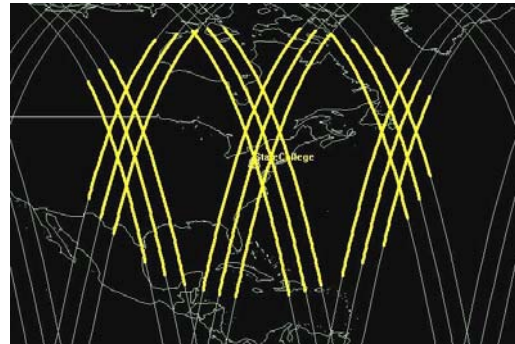
Figure 4. The typical coverage for a mid-latitude site with the satellite above the horizon indicates a couple of passes/day should be expected.
