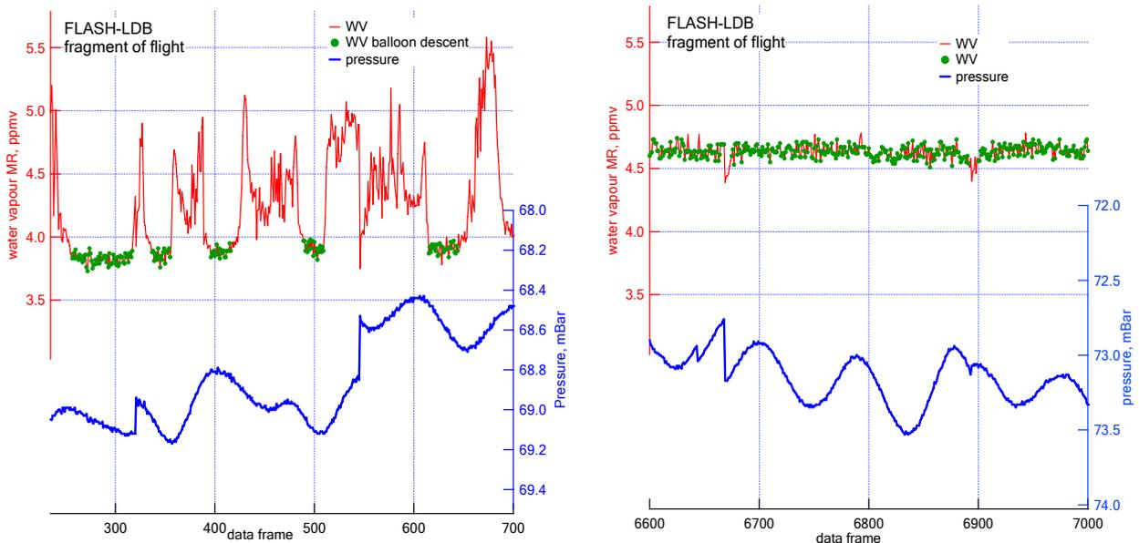
Figure 2. Water vapour and pressure from the two different flight fragments; first day of flight (left panel) and fifth day of flight (right panel). The contamination-free water vapour data are marked with green circles. The right axis (pressure) is reversed.
