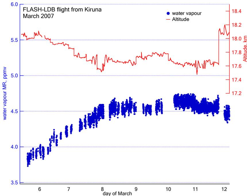
Figure 3. The results of water vapour mixing ratio measurements using FLASH-B in the long-duration balloon experiment. The balloon float altitude is plotted versus right vertical axis.
