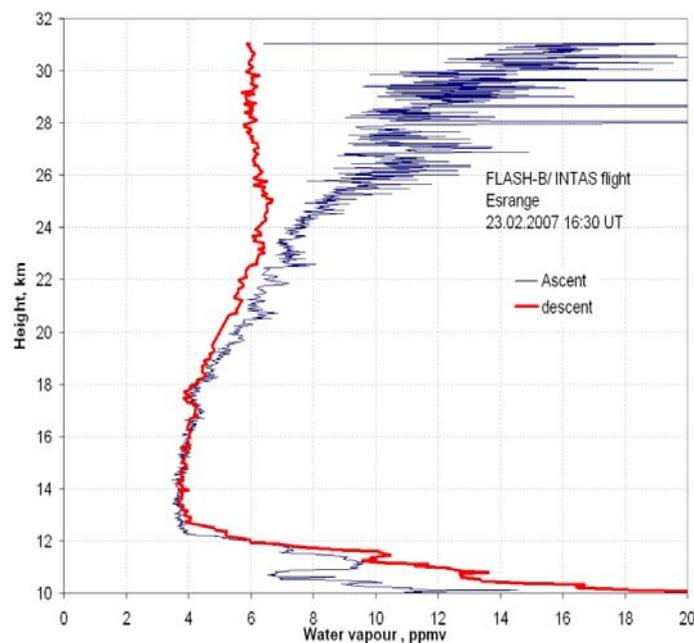
Figure 1. Vertical water vapour profiles obtained during in short-term balloon sounding conducted from Esrange on 23.02.2007.
