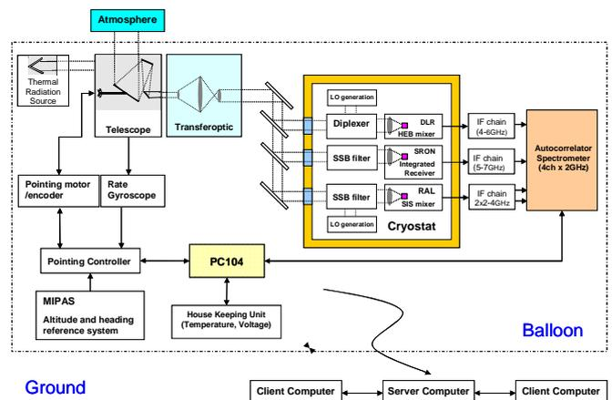
Figure 1: Block diagram representing TELIS instrument
