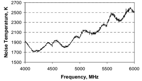
Figure 4: Double sideband noise temperature spectrum of 1.8 THz channel measured with the autocorrelator. LO was tuned at 1830.214 GHz.
