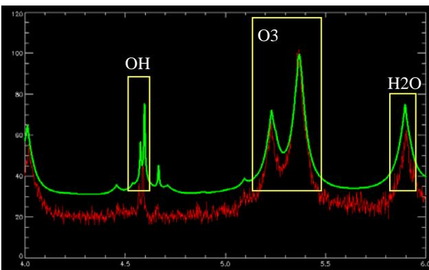
Figure 6: Comparison of the calibrated spectrum measured while the gondola was at 32.17 km and the simulation from the Hitran database. Integration time for complete limb sequence (18 different tangent heights) 30 minutes, 8:30 local time, latitude 66.25°, longitude 27.15°.
