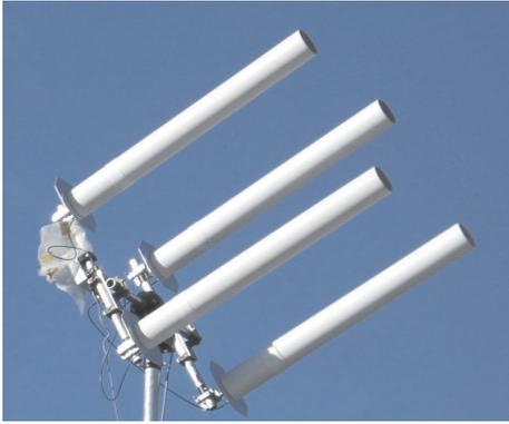
Figure 6. Receiving antenna for 869 MHz telemetry signal. The four tubes protect one helical antenna, each. The antenna mount is motorized to follow automatically the direction of the payload by evaluating the RS92's GPS data.
