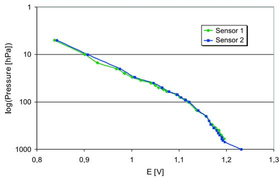
Figure 3. Sensor response at zero wind speed within a vacuum chamber at different pressures. The two different sensors show similar behavior with a changing slope around  $\sim 200$  hPa. The tests have been conducted with a 55P13 sensor (similar to 55P03 without gold-plated ends).
