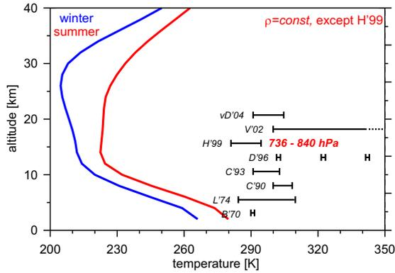
Figure 2. Typical temperature profiles for the mid-latitude troposphere and stratosphere (from [14]) compared to the temperature ranges for CTA calibration reported so far. Up to now there is no knowledge on CTA calibration at low temperatures. Additional uncertainties exist with respect to density effects. References for CTA data are given in the text.
