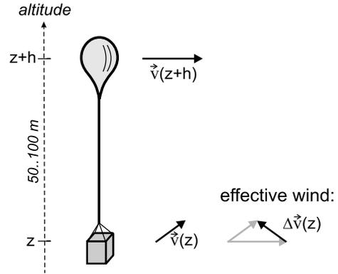
Figure 4. Schematic drawing of the principle of balloon borne wind turbulence soundings.
