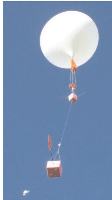
*Figure 5. Balloon and payload shortly after start. The rope is only slightly unwinded, yet. The lower red box contains the scientific payload.*
