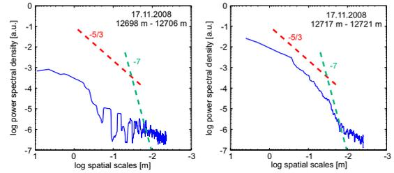
Figure 7. Frequency spectrum after FFT of a 8 m (4 m) data series. In the left figure the spectrum exhibits much less turbulence. The noise level is not totally flat due to some remaining spurious motions of the payload during this flight.
