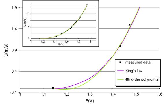
Figure 1. Calibration data for CTA sensor with fitted curves (King's law and 4th order polynomial). At low wind speeds the polynomial underestimates the true wind and gives partly even negative values.
