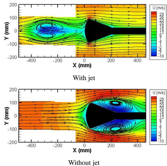
Figure 8. Jet/free-stream interaction in landing.
