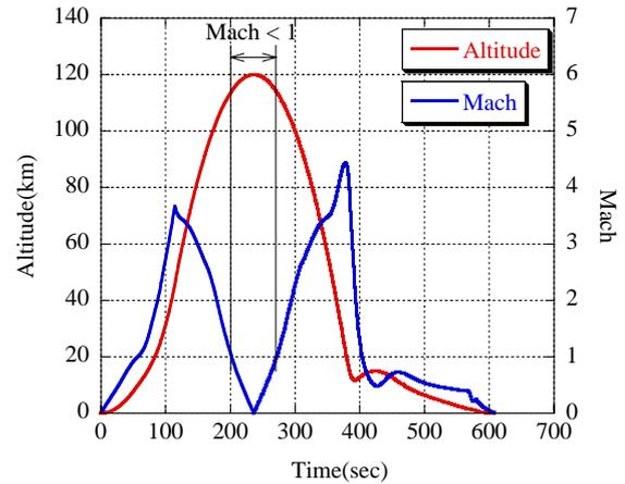
Figure 4. Flight profile: Altitude, Mach number.
