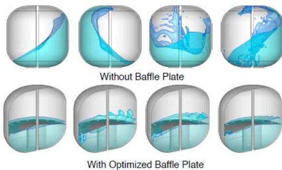
Figure 9. Sloshing simulation.
