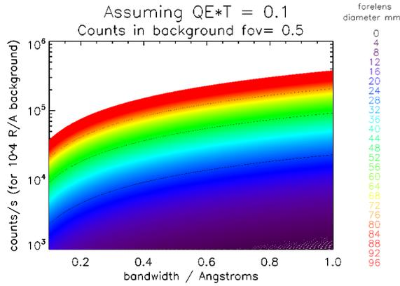
Figure 6. Photon counts for a background level of  $10^4$  R/Å as a function of the Fabry-Perot etalon bandwidth and light collecting diameter. Field of view is 0.5 degrees.
