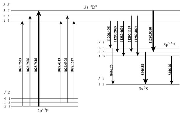
Figure 2. The primary path of Bowen fluorescence in OI 844.6 nm emission. [9]
