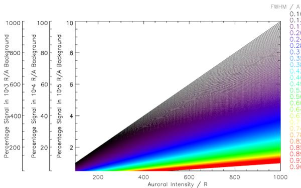
Figure 7. Ratio between counts per second produced from aurora 100-1000 R and by background levels of  $10^3$ ,  $10^4$  and  $10^5$  R/Å.
