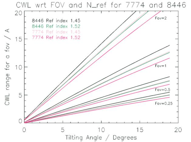
Figure 4. Spread of the central wavelength as a function of tilt angle and field of view for 777.4 nm and 844.6 nm for the refractive indices 1.44 and 1.52.
