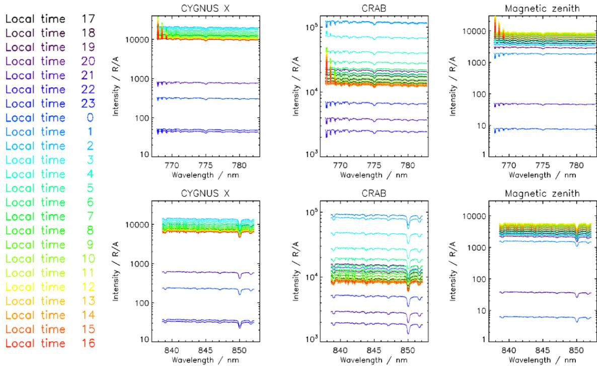
Figure 3. Theoretical sky background levels from the Modtran4 atmospheric model for the two target look directions as well as magnetic zenith for comparison.
