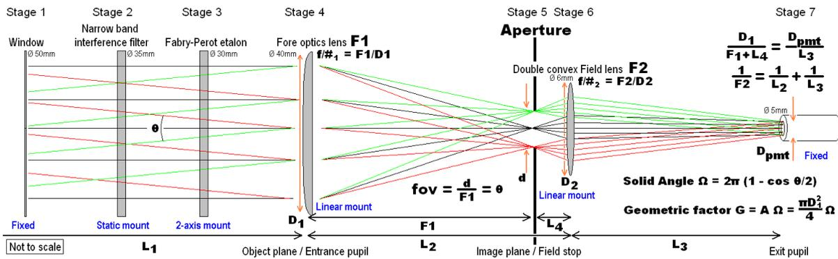
Figure 8. Optical layout. The values of the quantities are listed in Tab. 1.
