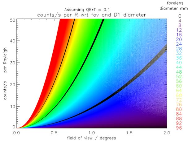
Figure 5. Number counts of photons per Rayleigh as a function of light collecting diameter and field of view on target lines of aurora. Diameters of 25, 50 and 75 mm are highlighted in black.
