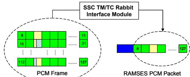
**Figure 6. Encapsulation of PCM Frames into RAMSES PCM Packets**
