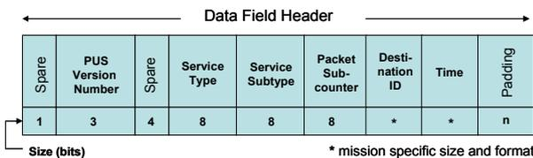
Figure 3. ECSS Data Field Header
