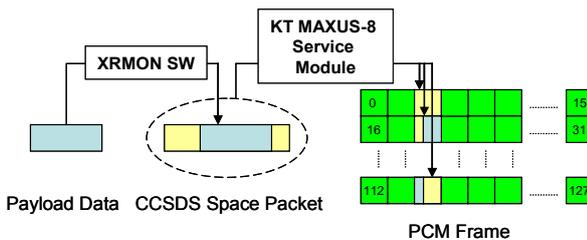
**Figure 5. Encapsulation onboard of payload data**
