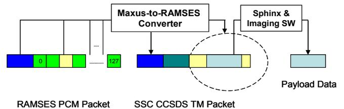
**Figure 7. Extraction of CCSDS Space Packets and Payload Data**
