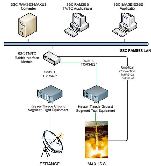
Figure 4. Ground segment setup for the XRMON-diff experiment
