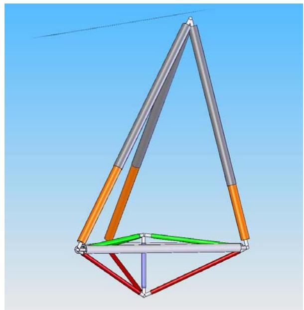
Figure 2. A different beam length makes the center of the mass and the rotation axis overlap without adding extra weight
