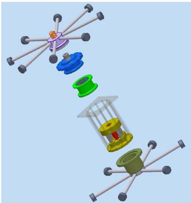
Figure 3. The current features of the pivot , which are capable of suspending gondolas up to 2500kg of weight are sketched in an exploded view
