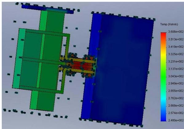
Figure 6. Thermal analysis of an example of pure hydrogen FC assembly (without taking into account the valve system, reactant flux control and by product. Both stack and tanks are in the correct operating range.
