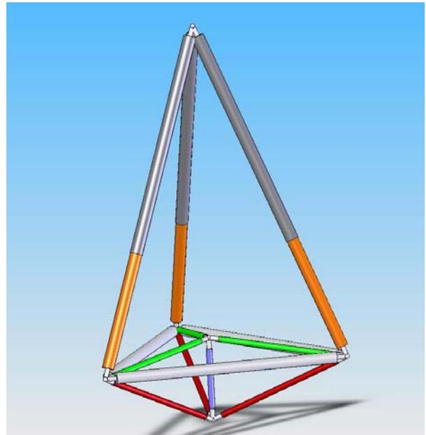
Figure 1. Modular structure in which each beam undergoes only tensile or compression stress.- In this way we can minimize the weight of the gondola
