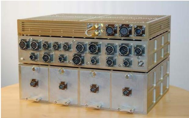
This year a modern TM system for payload purposes has been qualified and become operational. The system is a 2 Mbps data link with Ethernet interface and consists of 4 airborne units and 2 mobile ground stations.
