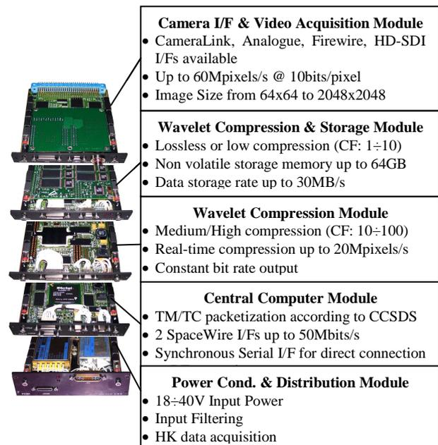
Figure 2: Typical H<sup>2</sup>VMU Arrangement
