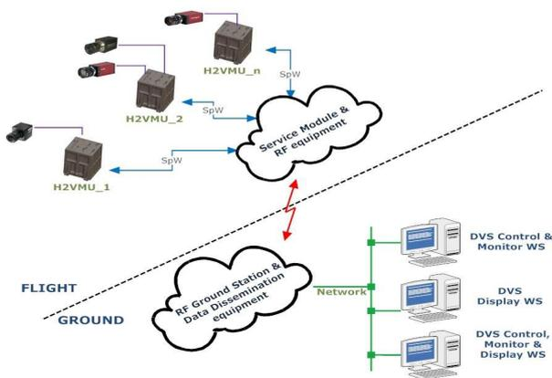
Figure 1: DVS Concept in Sounding Rockets
