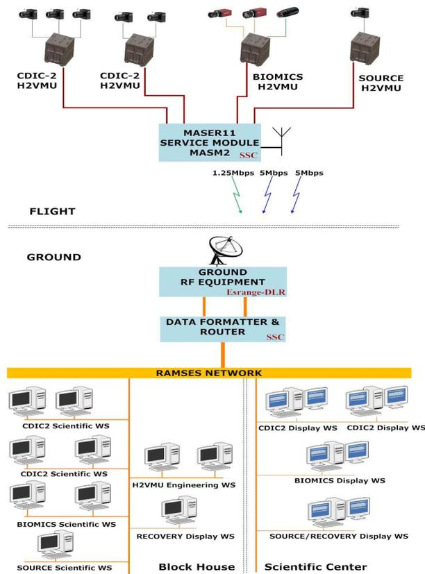
Figure 3: Maser11 DVS Configuration
