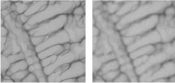
Figure 3. Focus spot size effect on image quality: left 3 $\mu\text{m}$ , right 7  $\mu\text{m}$
