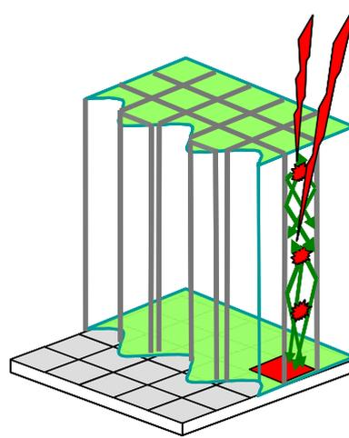
Figure 5. Structured scintillator principle
