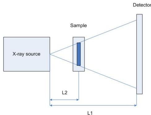
Figure 2. geometrical magnification of object on detector
