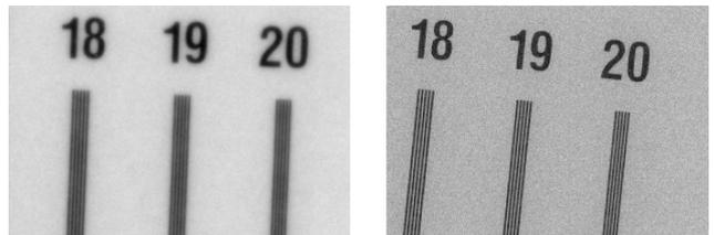
Figure 6. Comparison of image from needle type scintillator and structured scintillator
