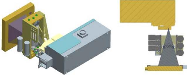
Figure 9. XRMON-diffusion experiment x-ray path: side view / top view
