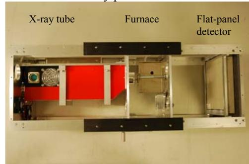
Figure 8. XRMON-foam experiment x-ray chamber (opened)
