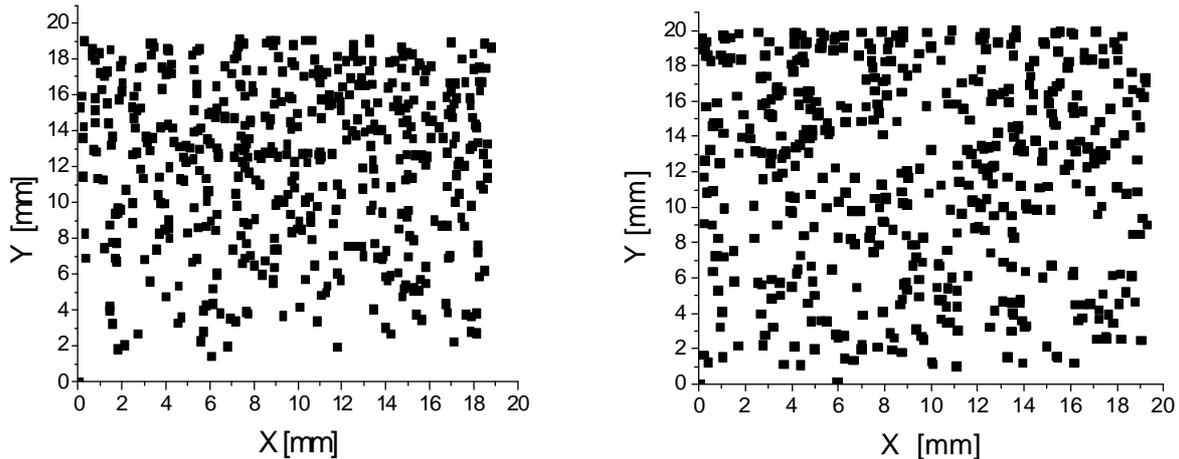
Figure 6. Cell wall rupture map of the Thixo AlSi6Cu4 foam in the liquid state during almost 4 minutes under gravity (left) and during MASER 11 (right) extracted from the sequence of X-ray images.
