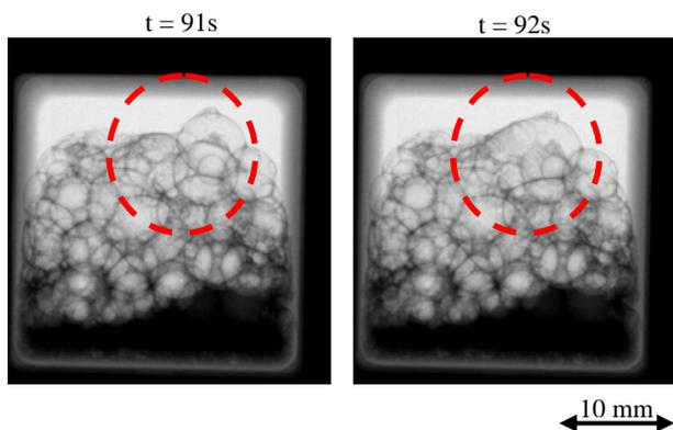
Figure 4. Cell wall rupture and consequent coalescence of 2 bubbles on the top of a liquid Thixo AlSi6Cu4 foam under 1.8 g. Broken circles show the region of interest.
