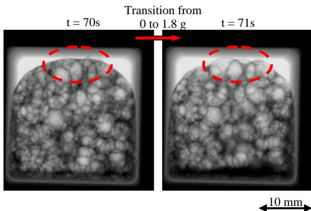
Figure 3. Liquid flow from top to bottom during transition from 0 to 1.8 g in a Thixo AlSi6Cu4 foam. Red ellipses denote the region of interest.
