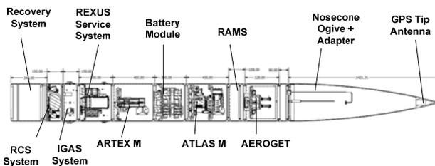
Figure 3. Sketch of the MAPHEUS-1 Payload [7]
