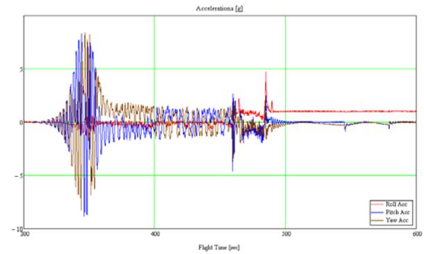
Figure 11. Roll, Yaw and Pitch Acceleration during Re-entry as Function of Flight Time
