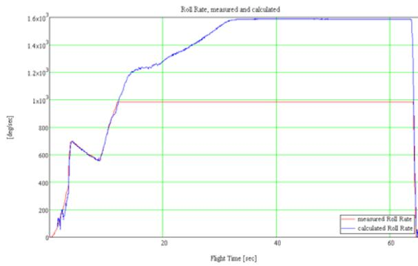
Figure 9. Roll-Rate during Ascent Phase as Function of Flight Time
