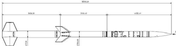
Figure 1. MAPHEUS-1 two-stage unguided solid propellant sounding rocket [7]
