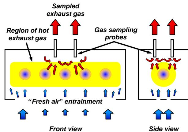
Figure 5. Sectional views of the combustion chamber during the exhaust gas sampling.
