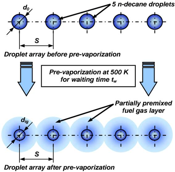
Figure 1. Schematic on fuel pre-vaporization of a linear droplet array.
