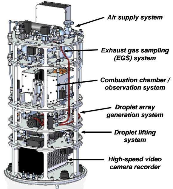
Figure 2. "Droplet Array Combustion Experiment Unit" (DCU), core section of the TEXUS experiment.
