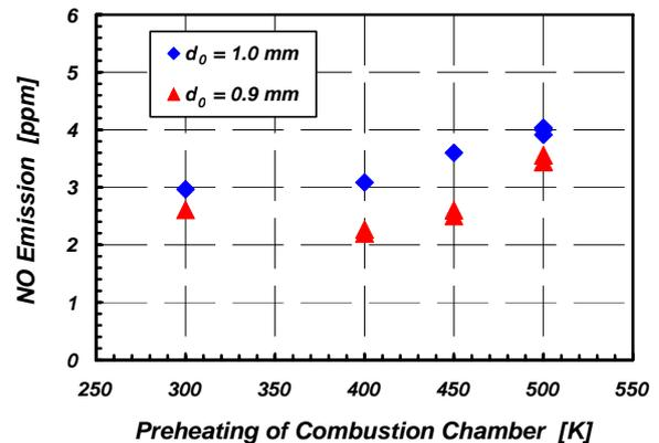
Figure 7. Precursor drop tower experiments with different droplet sizes and preheating levels.
