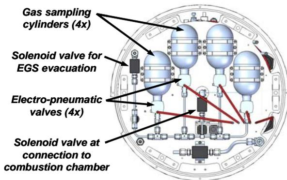
Figure 4. Exhaust gas sampling (EGS) platform with coated gas sampling cylinders and supply units.
