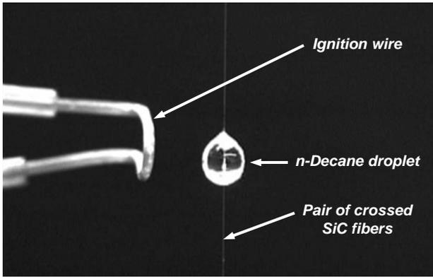
Figure 3. Ignition wire (left) and n-decane droplet, suspended on SiC fibers (middle).
