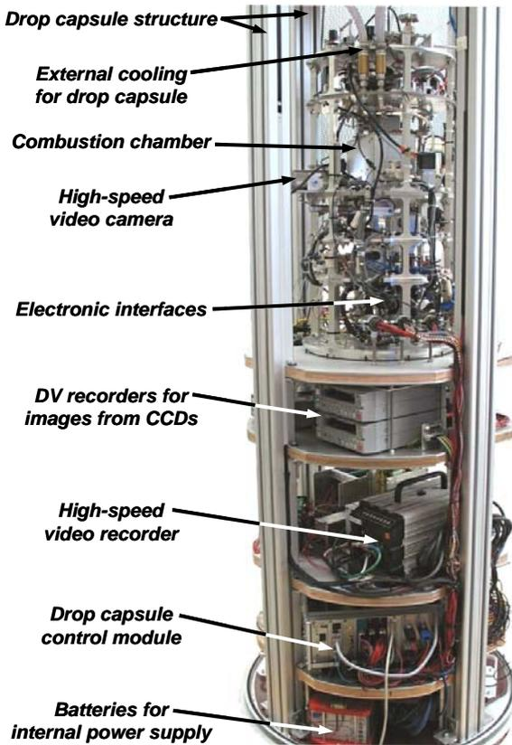
Figure 6. Drop tower setup with the DCU being integrated in the upper half of the drop capsule.
