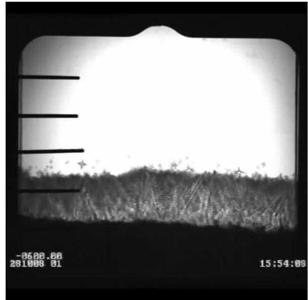
Figure 13. Many growing equiaxed grains ahead of the columnar solid-liquid interface at  $t = 1541$  s
