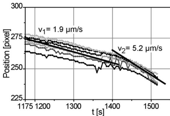
Figure 8. Solid/liquid interface positions evaluated from macro images while increasing the cooling rate
