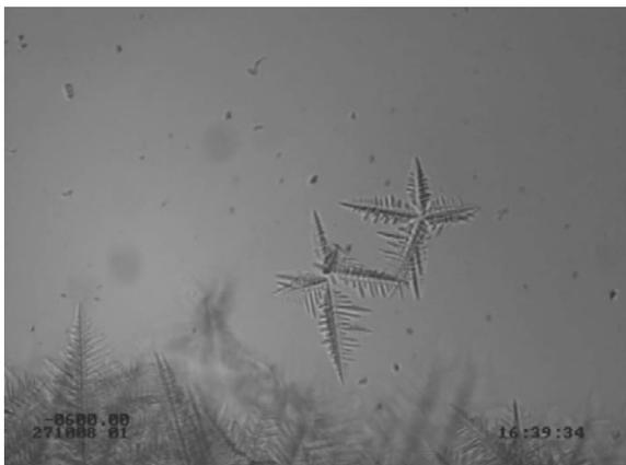
Figure 14. Growth and movement of equiaxed grains in gravity; time intervals between successive images  $\Delta t = 58$  s and  $\Delta t = 50$  s; field of view  $2.1 \times 1.7$  mm<sup>2</sup>
