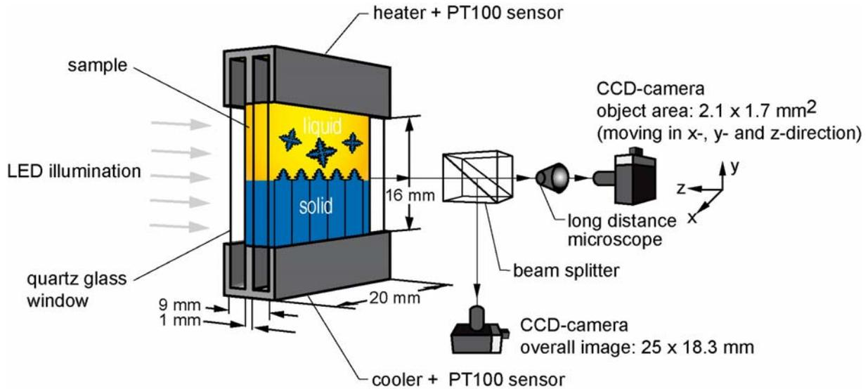
Figure 1. Sketch of the experiment chamber and the optical system
