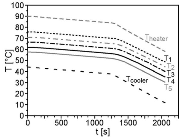
Figure 4. Heater and cooler temperatures and temperature profiles inside the sample (T1 to T5)
