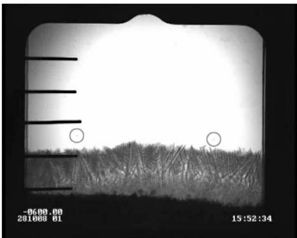
Figure 12. Nucleation of two equiaxed grains (marked by circles) in the undercooled melt at  $t = 1450$  s
