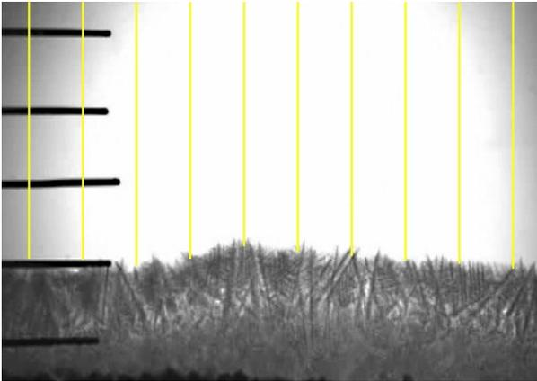
Figure 6. Macroscopic image to determine the interface velocity at different lateral position
