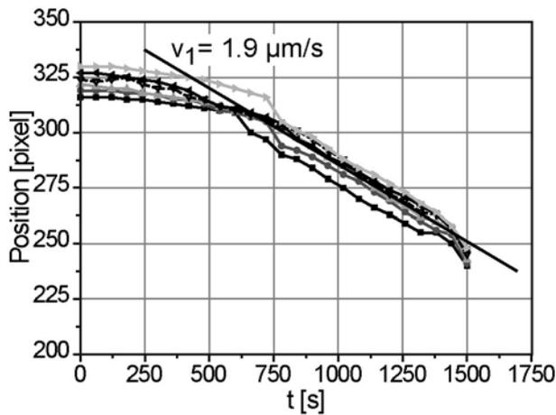
Figure 7. Solid/liquid interface positions evaluated from macro images for the cooling rate 0.28 K/min
