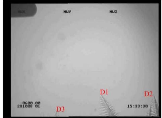
Figure 9. Detail image showing the growth of single dendrites at  $t = 300$  s
