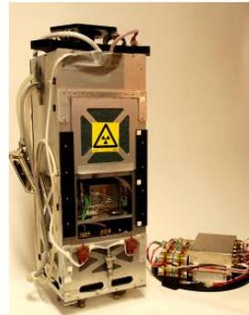
Figure 8. The X-ray tight damped inner structure to the left, electronics deck to the right. Access hatch is open, showing the furnace inside
