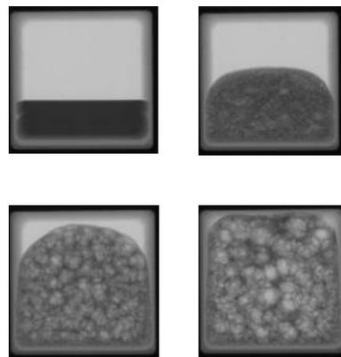
Figure 9. Foam generation in XRMON during flight
