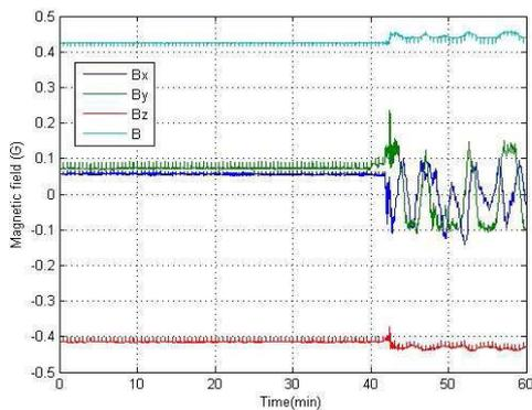
Figure 8 – Magnetometer Measurements during Ascending Phase
