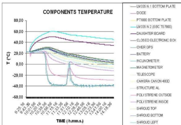
Figure 5- Results of the AURORA experiment thermal-vacuum test
