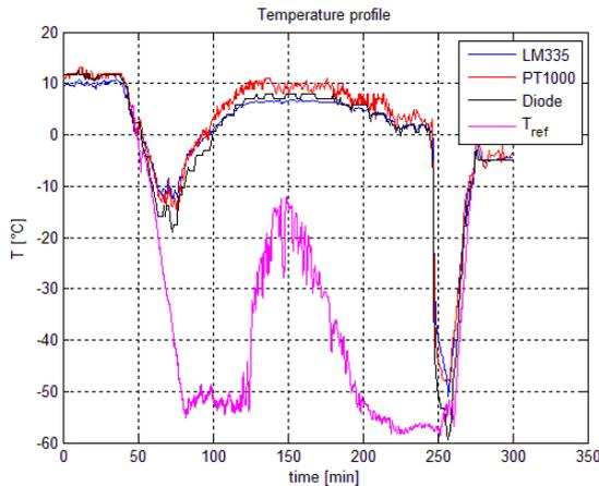
Figure 18- Compared temperature measurements
