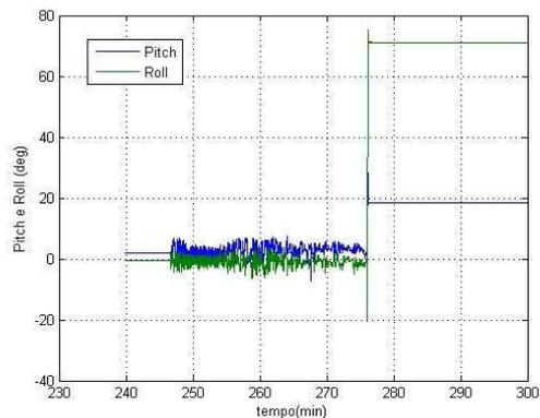
Figure 12- Inclinometer Measurements during Ascending Phase
