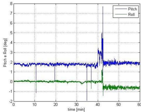
Figure 11 - Inclinometer Measurements
