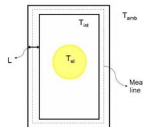
A preliminary thermal test was conducted at university [5], using a conditioned cell. Results conducted to have a thermal protection of 9 cm of polystyrene to guarantee temperature range functioning for the motherboard.
