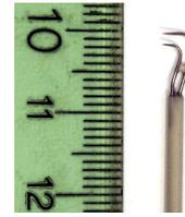
Figure 3. Sensor probe with the platinum-plated wire (Type 55P03, Dantec Dynamics) which has a diameter of 5  $\mu\text{m}$  and a length of 1.25 mm. The wire is welded to the prongs.
