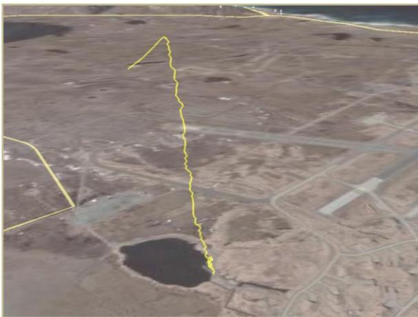
Figure 5. GPS trace of descending CanSat illustrated in Google Earth
