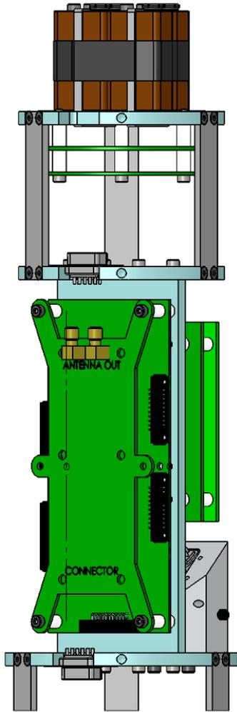
Figure 3, Batteries, electronic section and housekeeping
