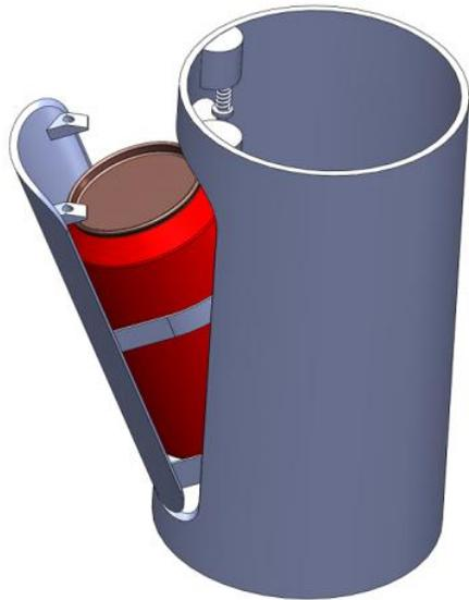
Figure 6, First Concept for releasing a CanSat [10]
