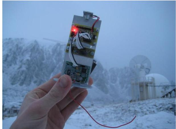
Figure 5, The inside of a CanSat kit used in the CanSat competition (R. Vanderberg, NAROM) [9]
