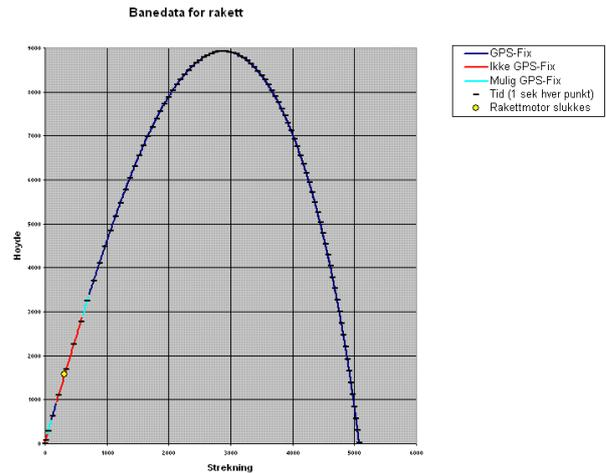
Figure 4, GPS lock vs trajectory simulation [7]
