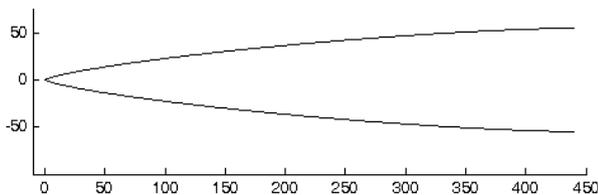
Figure 1, Von Karman shape nosecone, scale in mm
