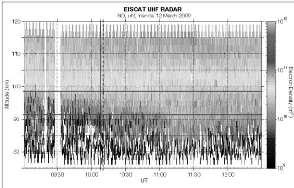
Figure 5. Electron density measurements during the REXUS 6 launch. The lift-off at 10:08 UT and the rocket apogee at ~10:10:40 UT are marked by vertical solid and dashed lines, respectively. The altitude region scanned by the trisatic intersection point is bounded by horizontal lines.
