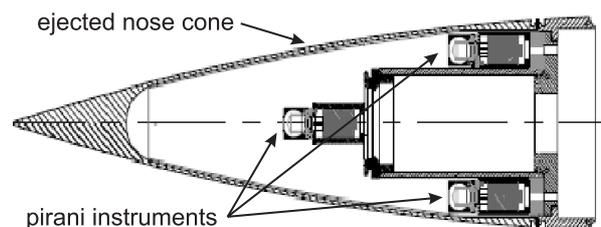
Figure 4. PIRANI sensors on the REXUS payload
