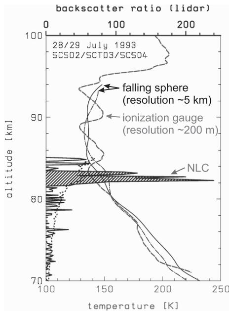
Figure 1. Near common volume measurements of a noctilucent cloud (NLC) by lidar and temperature profiles by different sounding rocket techniques. The dashed line shows a high resolution measurement with an ionization gauge, the solid and dash-dotted lines show accompanying measurements obtained with the falling sphere technique. After [RLM<sup>+</sup>02].
