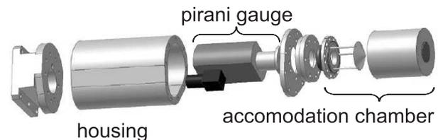
Figure 2. Drawing of the Pirani instrument that includes complete electronics, accommodation chamber (Pitot-chamber), and housing (including mounting).
