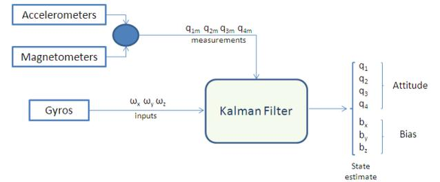
Figure 11. Kalman filter for AHRS
