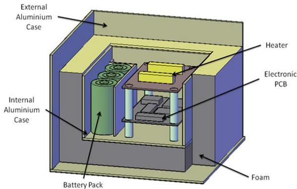
Figure 3. Mechanical design
