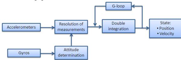
Figure 5. Inertial navigation process
