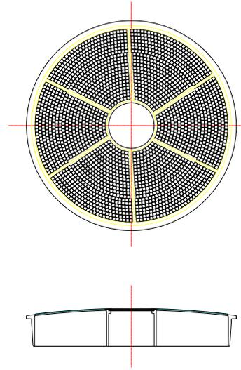
Figure 3. The HAXTEL-B Laue lens subsystem.
