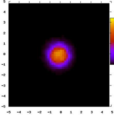
Figure 6. The expected HAXTEL-B Laue lens image of an on-axis source (PSF) for the proposed 6 m focal length configuration; both scales are in cm.
