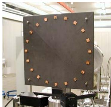
Figure 1. The first Laue lens prototype model developed at the LARIX facility in Ferrara (Italy).
