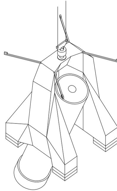
Figure 5. A possible flight configuration for the HAXTEL-B balloon borne payload.
