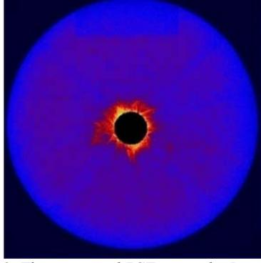
Figure 2. The measured PSF using the Laue PM compared with the ideal one (black circle) obtained with a Monte Carlo code by assuming a perfect positioning of the Cu tiles in the lens.
