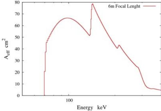
Figure 7. The HAXTEL-B Laue lens effective area as a function of energy
