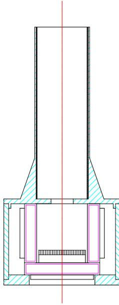
Figure 4. The HAXTEL-B focal plane detector scheme.
