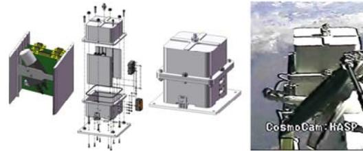
Figure 3. HEMI Pathfinder Instrument Design (left) and in Flight on HASP (right)
