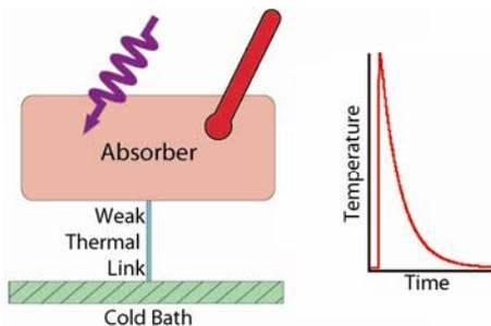
Figure 2. The working principle of a microcalorimeter.
