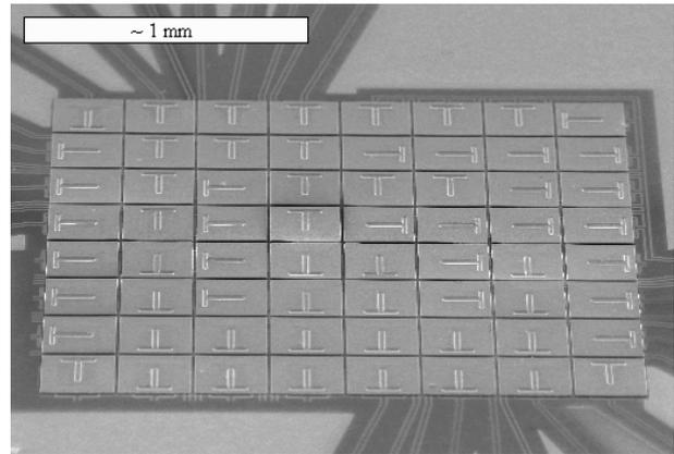
Figure 3. A GSFC  $8 \times 8$  TES Microcalorimeter Array.
