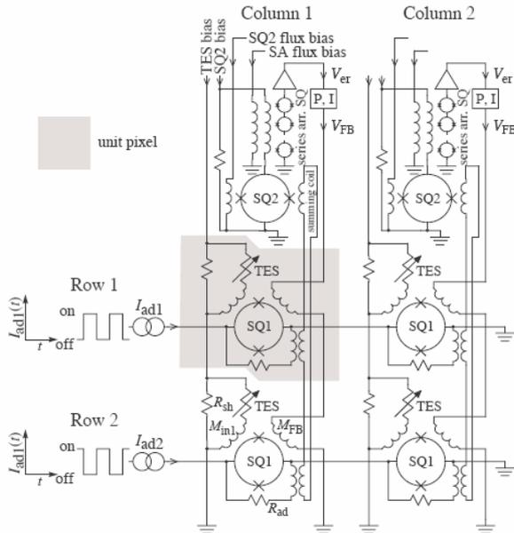
Figure 4. Schematic of the Time-Division SQUID Multiplexing System.
