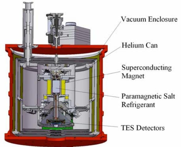
Figure 5. The Micro-X Cryogenic System.
