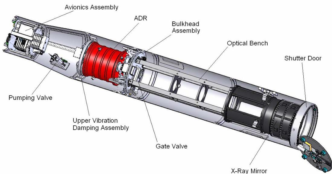
Figure 7: The Micro-X Science Instrument.
