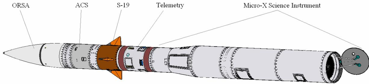
Figure 6: The payload section of the Micro-X sounding rocket.
