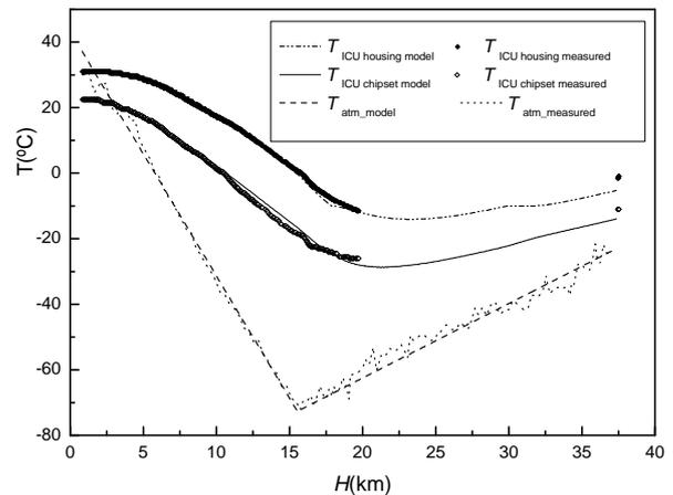
Figure 4. Temperature,  $T$ , versus altitude,  $H$ , of the box housing and inner chipset (measured and model results). Atmospheric air temperatures (measured and linear approach) are also indicated.
